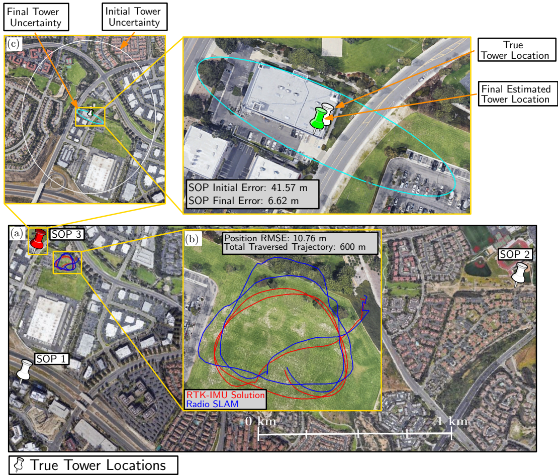
Figure 2.5: (a) Experiment layout containing the true locations of each SOP tower and the two UAV navigation solutions. (b) UAV trajectory comparison between the RTK-IMU navigation solution (red) and radio SLAM (blue). (c) Initial and final position estimates with their associated north-east uncertainty ellipse for SOP tower 3. Map data: Google Earth.
