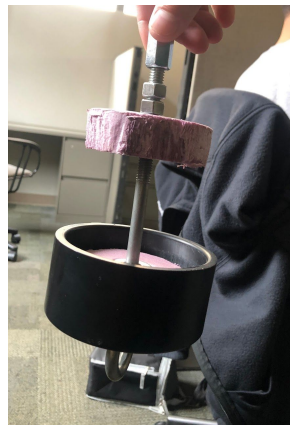
Figure 3a: Coupling mechanism attached to hook's shaft
